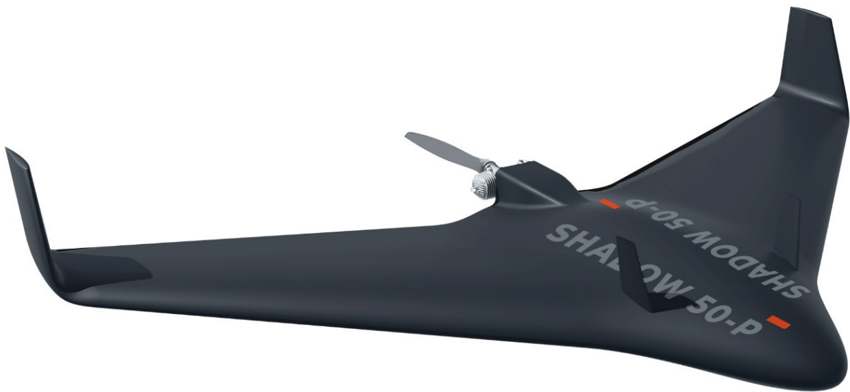
The SHADOW 50, a fixed-wing, turbojet UAV
