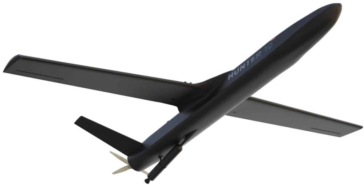
The HUNTER 10, a fixed-wing, tube launched UAV
