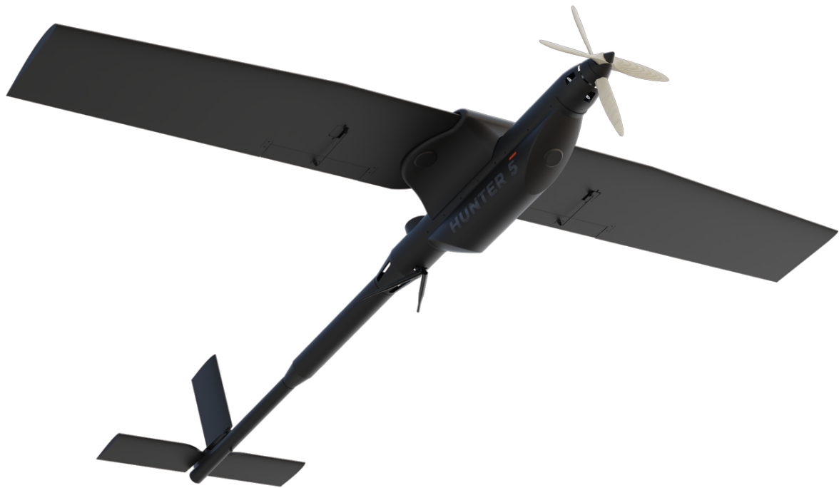
The HUNTER 5, a fixed-wing, propeller engine UAV
