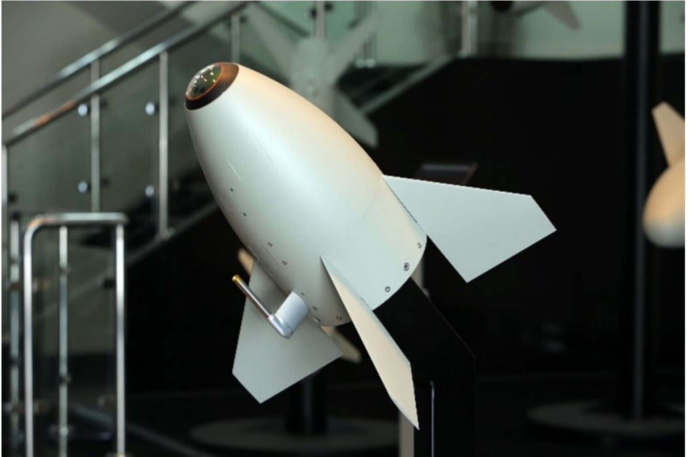
An AL TARIQ front component with a semi-active laser
